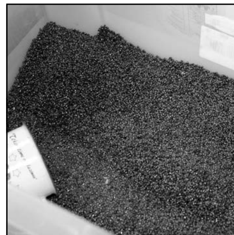
Figure 6: Copper shot after use.
