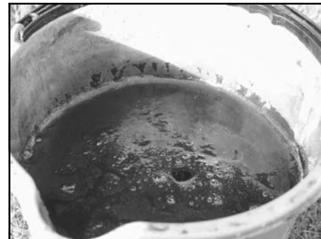
Figure 5: Black, foamy liquid generated by the tumbling.
