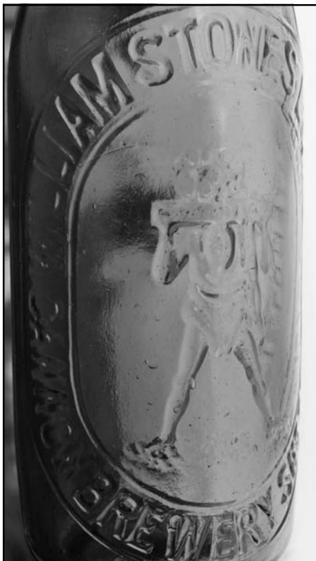
Figure 3: An acid dipped bottle: shiny finish but with a waxy “orange peel” surface complete with pits and scratches.
