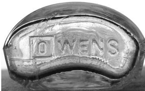
Figure 9: Box-O creating the first letter of “OWENS” on a drug store bottle base (Lockhart)
