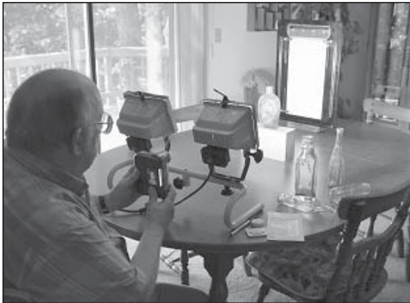
My photographic set-up on my wife's dining room table. I'm shooting the camera from in between the work lights with the bottle about 18-inches in front of the light source.
