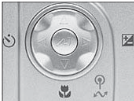
Figure 4: The ability to focus on objects close at hand is usually denoted by a small tulip icon, as seen on the back of this Nikon.
