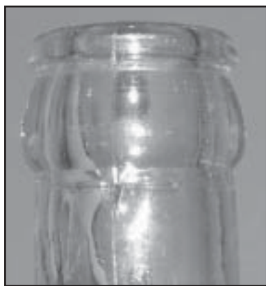
Figure 2: Root Semiautomatic Bottle Finish
