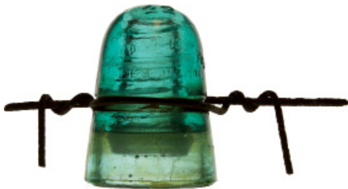
This crown-embossed “beehive” was manufactured between 1884 and 1890. This photo demonstrates how the tie wire was used to attach the iron telegraph wire to the insulator.
