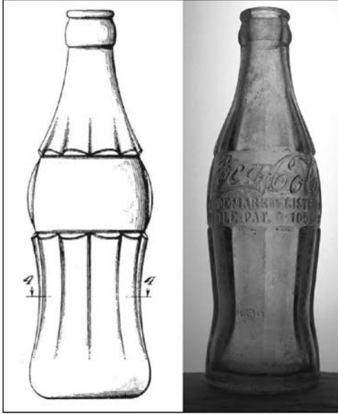
Figure 25 – Comparison of 1937 patent drawing (D-105523) with actual bottle
