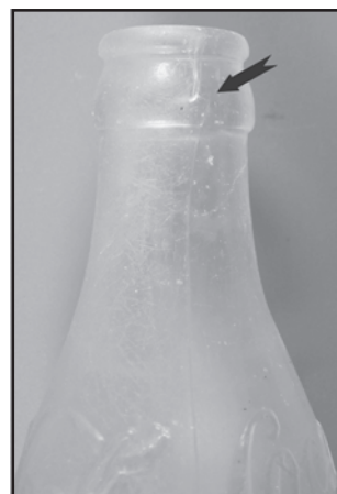
Figure 10: Side Seam – Straight-Sided Coke Bottle
