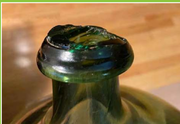
Figure 9: The Dame Jeanne's peculiar and distinctive snapped-off top and applied-ring lip.
